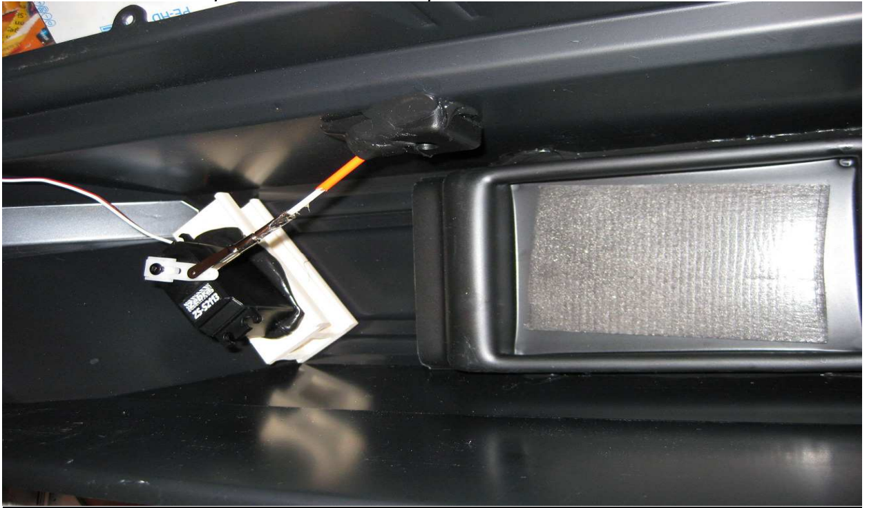
Illustration: Servo operation of 1 feed flap with Bowden cable
